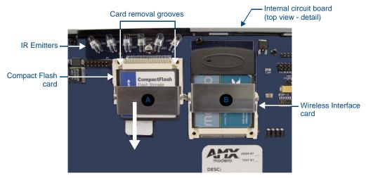
FIG. 6 Location and orientation of the Compact Flash cards (both MVP panels)
